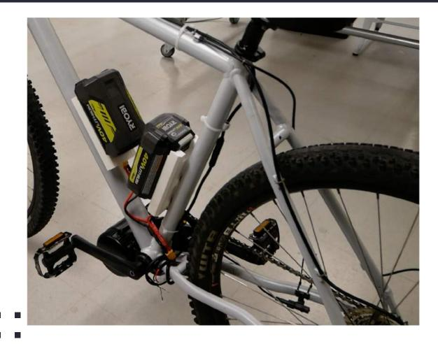
Our system consists of two RYOBI 40V 4Ah lithium ion batteries attached to the ebike via mounts we designed that connects in parallel to the motor via a Y-harness.
