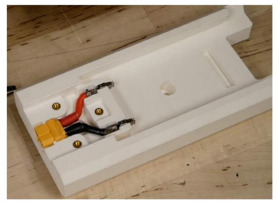
The mount features rails for the battery to slide into, a slot for the battery's latch to lock into, two mounting holes to attach the mount to the bike, geometry to hold the internal harness in place and mounting points for a wire cover.
