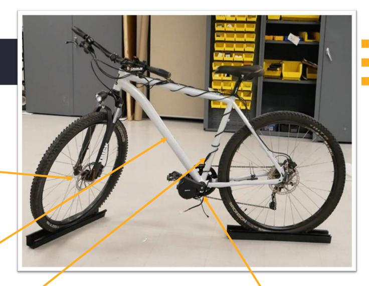
Each set of water bottle bosses will allow for 1 battery to be mounted to the bike frame. If two batteries are desired for operation, water bottle bosses located on both the down tube and seat tube are preferred.
